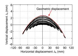
(a) Displacement orbit of Specimen L11C
