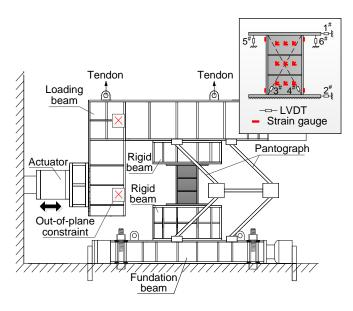
Fig. 4. Test setup and instrumentation
