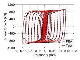
Fig. 12. Comparison between FE analysis result with test data for Specimen L11
