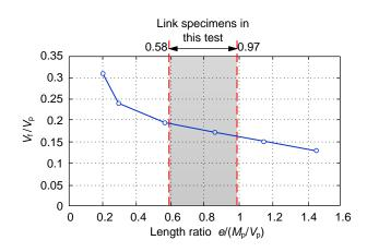
Fig. 11. Flange contribution on shear strength
