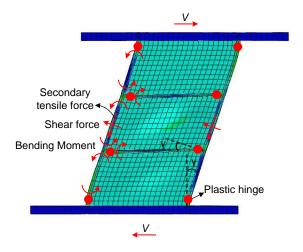
(b) Inner forces in flanges (with respect to coordinate system of deformed configuration)
