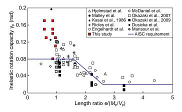
Fig. 8. Inelastic rotation capacity versus length ratio of shear links
