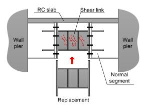
Fig. 1. Schematic drawing of replaceable steel coupling beam
