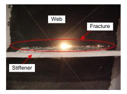
(c) Web fracture (Specimen L12)
