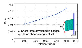
(a) Shear force in flanges (with respect to coordinate system fixed to original configuration)
