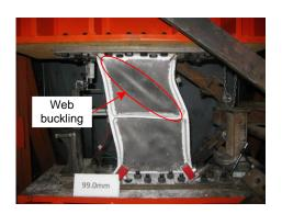
(a) Web buckling (Specimen L13)
