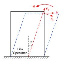
(b) Force decomposition at large inelastic
