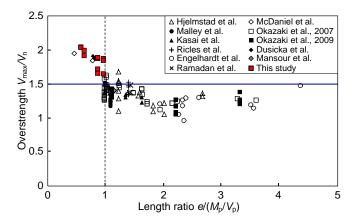
Fig. 9. Overstrength factors of link test data
